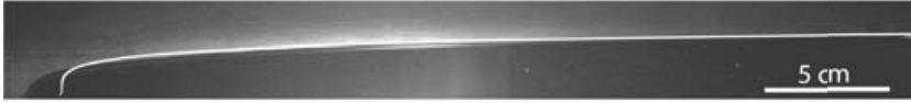
FIGURE 5. Photograph from the top of the gravity current propagating 95 cm from right to left along a horizontal semicircular channel, 47 s after 341 \text{ cm}^3 of glycerine with a viscosity of 3.22 \text{ cm}^2 \text{ s}^{-1} was released. The solid white line marks the fluid boundary as predicted by theory.
